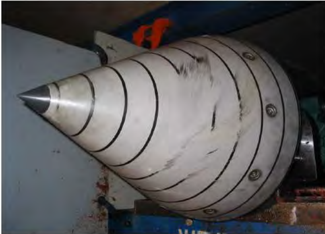
Figure 13. The spinner cone immediately after impact with the 6.0lb bird.
